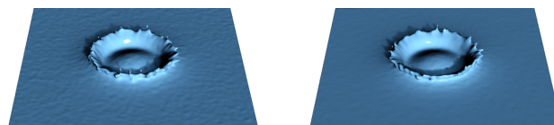
Fig. 6. Drop falling into a quiescent pool of water simulated at CFL = 15. Adaptive \gamma attenuation (right) reduces noise in the calm water surface region while preserving the splash details.
