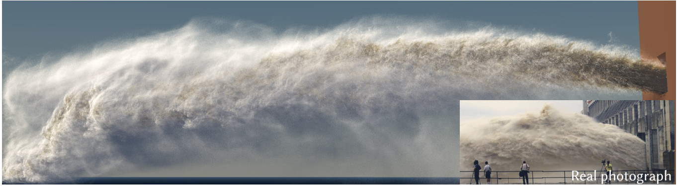
Fig. 3. Phase-Field-FLIP simulation of a large dam discharge showing violently turbulent water-air interaction induced by a powerful water jet at high speed ( \approx 40\text{m/s} ). A real photograph of a dam discharge event at similar scale (Three Gorges Dam, China, © Picture Alliance) is included in the lower right corner. No effort was made to tune the simulations for the exact conditions of the reference, and no turbulence enhancement or post-processing effects were applied. The effective resolution is 2048 \times 1024^2 for the pressure and 8192 \times 4096^2 for the liquid surface and spray density, with \approx 40\text{s} simulation time per time step.
